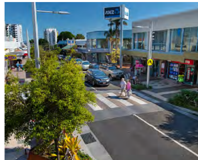
Raised pedestrian crossings
